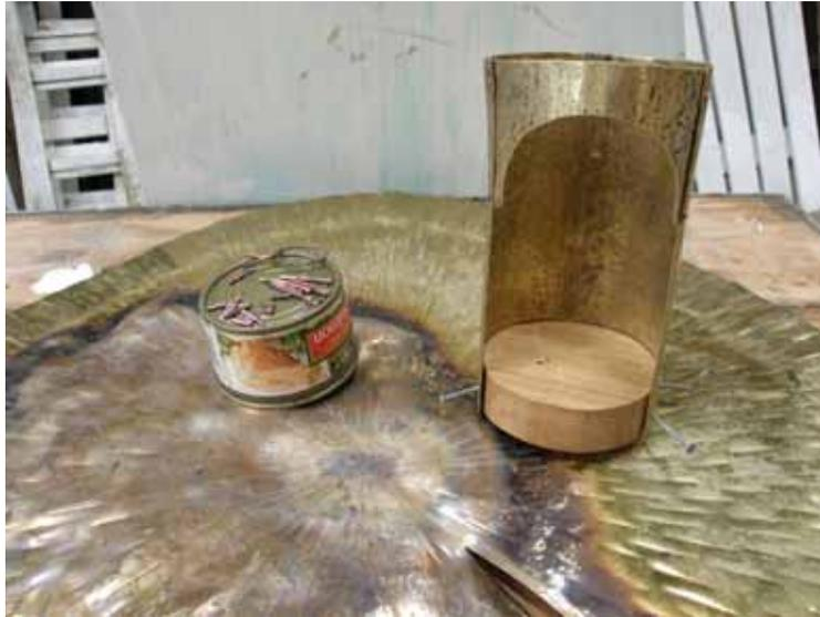
To the left are the copper rivets made from a heavy piece of copper wire melted at one end. The body made from three pieces of brass sheet and the wooden base.
