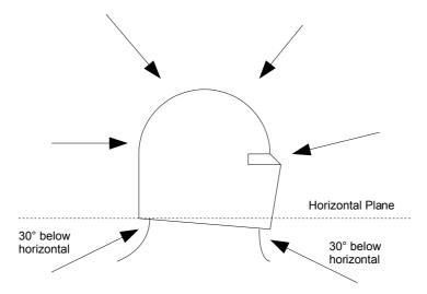
This includes eye protection. Any eye slots or openings must be covered by 1.6mm diameter heavy mesh or 1.6mm thick perforated steel with holes no larger than 5mm and 50% or less open area. Some examples are shown below:
