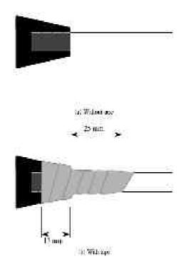
To allow inspection of possible punch-through the face of the blunt must not be covered.
