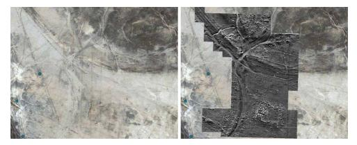
Figure 3: Left: IKONOS satellite image September 2001. Detail of the southern area. Right: Compilation of the satellite image with the magnetograms from March 2001 and 2002. Caesium magnetometry, Scintrex Smartmag SM4G-special, sensitivity 0.005 nT, dynamics -+12.00 nT in 256 grey scale (white/black), raster 0.5 x 0.1 m (interpol. 0.25 x 0.25 m), 40m grid.
