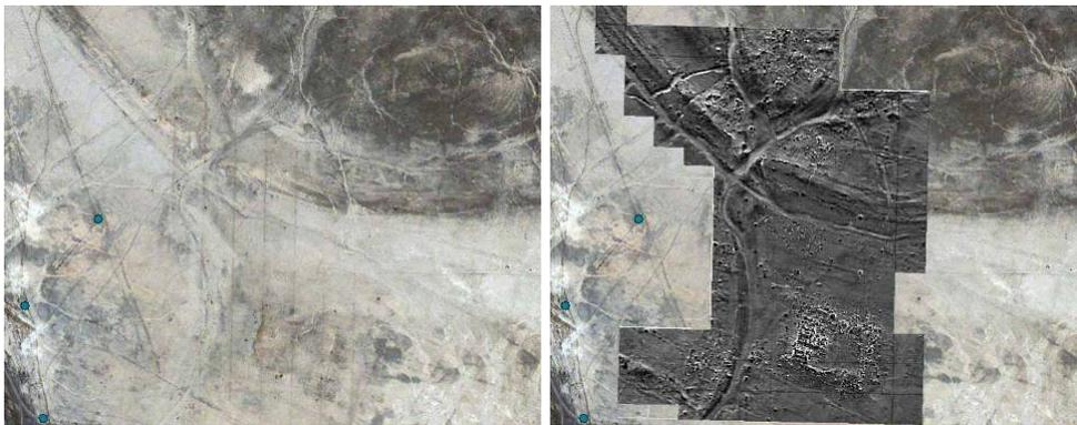
Figure 3: Left: IKONOS satellite image September 2001. Detail of the southern area. Right: Compilation of the satellite image with the magnetograms from March 2001 and 2002. Caesium magnetometry, Scintrex Smartmag SM4G-special, sensitivity 0.005 nT, dynamics  $\pm 12.00$  nT in 256 grey scale (white/black), raster 0.5 x 0.1 m (interpol. 0.25 x 0.25 m), 40m grid.
